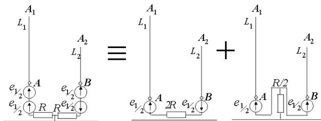
Fig. 6. To a calculation of two radiators in a near region
