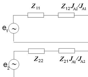
Fig. 4. The equivalent circuit of two coupled radiators
